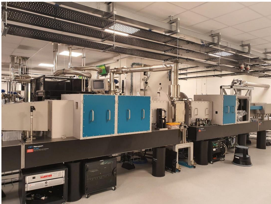
Figure 22: 100 J blast shields and amplifier head
