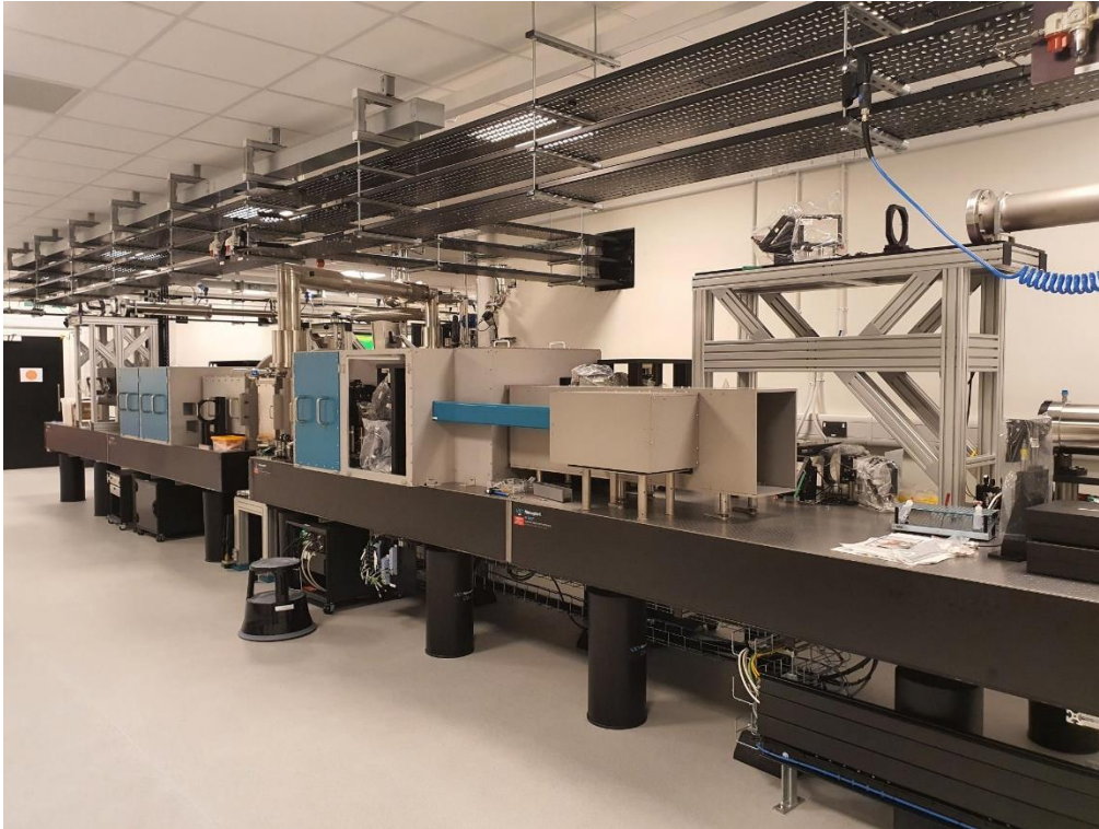
Figure 23: The 100 J beam transport to the Ti:Sapphire room
