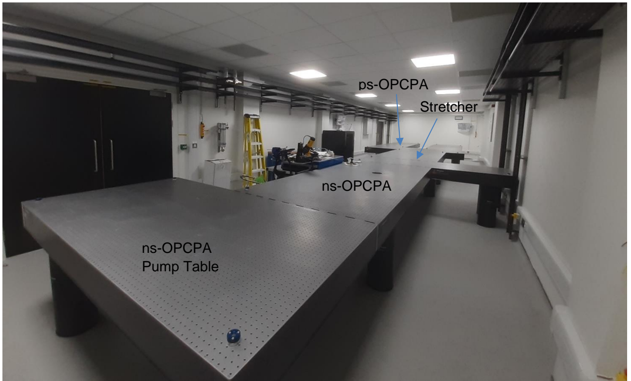
Figure 5: Photograph of the EPAC Front End Room in March 2023, when the main optical tables were installed
